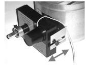
The bracket allows the actuator to be positioned on the shaft up to 2" above the damper to compensate for insulation that might be under it.
